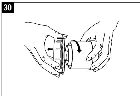
**!** Placing granules in the center of the cartridge allows them to escape in the unit or to clog the unit. The unit will no longer operate properly and the granules need to be cleaned out thoroughly.
