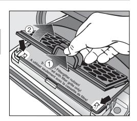
■ Insert a new Air Clean exhaust filter.
